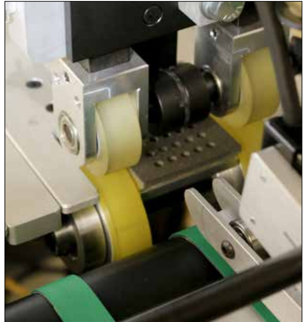
Adjustable feed rollers and vacuum plate.
