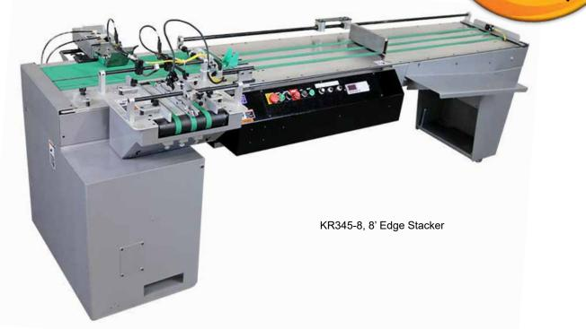
An all -new concept in mail handling, the KR345 takes hassle out of sorting and traying mail. Part shingle conveyor, part edge stacker, the KR 345 combines the advantage of each system into a simple, laborsaving unit.
