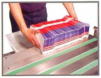
Fill trays in one motion by sliding bundles off the side of the conveyor.
