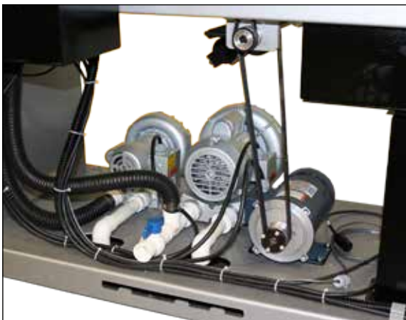
Base mount motor and pump reduces vibration.
