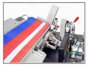
You don't need to buy another friction feeder with the KR 533. Angled brackets allow you to rotate the KR 533 matching the angle of your friction feeder.
