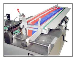
Adjust the table to a horizontal position and use the KR 533 with your shuttle feeder.
