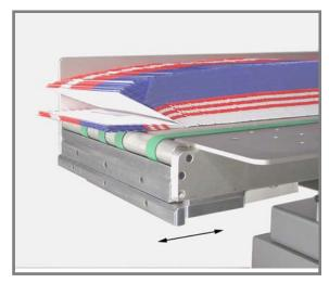
The KR 533's jogger assembly conditions material in the hopper improving feeder consistency
