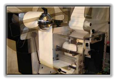
Run 3" wide labels on the standard KR540. Even wider labels are possible using the optional 5" wide label kit.
