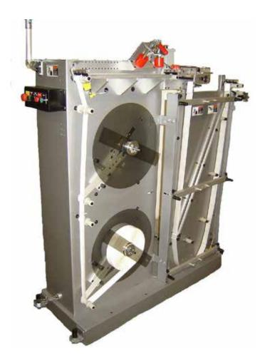
The KR565 is equipped with a low label strobe and features clamps to secure label during application of splicing tape. The operator completes the changeover by reloading the empty station and resetting the system for the next changeover.
