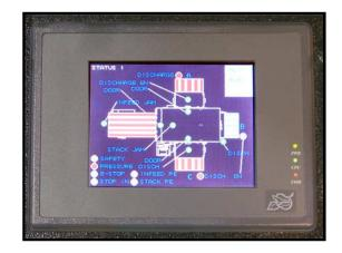
The control panel's graphical display indicates system status simplifying setup and maintenance.
