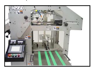
The receding lift table helps maintain stack integrity by minimizing the distance stacks drop between compensation cycles.
